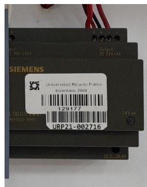
Figure N° 4: Stabilized Power Supply LOGO! Power 24 V / 4 A Source: Own
