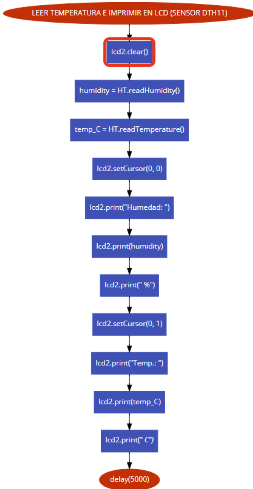
Fig. 4. Flowchart to detect humidity and temperature of the DTH11 sensor.
