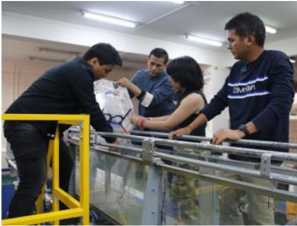
Figure 8: Placement of the prototype culvert in the variable slope canal variable slope channel Source: Own elaboration
