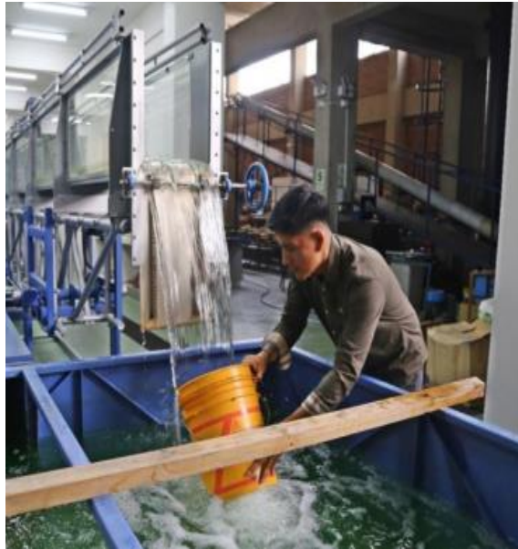
Figure 12: Application of the volumetric method
