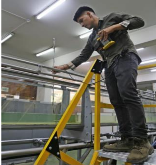
Figure 10: Placement of current meter to calculate water velocities Source: Own elaboration
