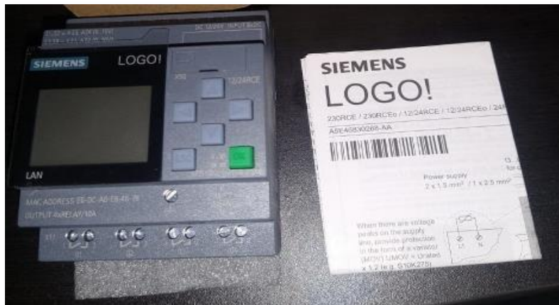
Figure 28: PLC controller logic
