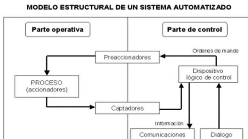
Figure 1: Structural model of an automated system
