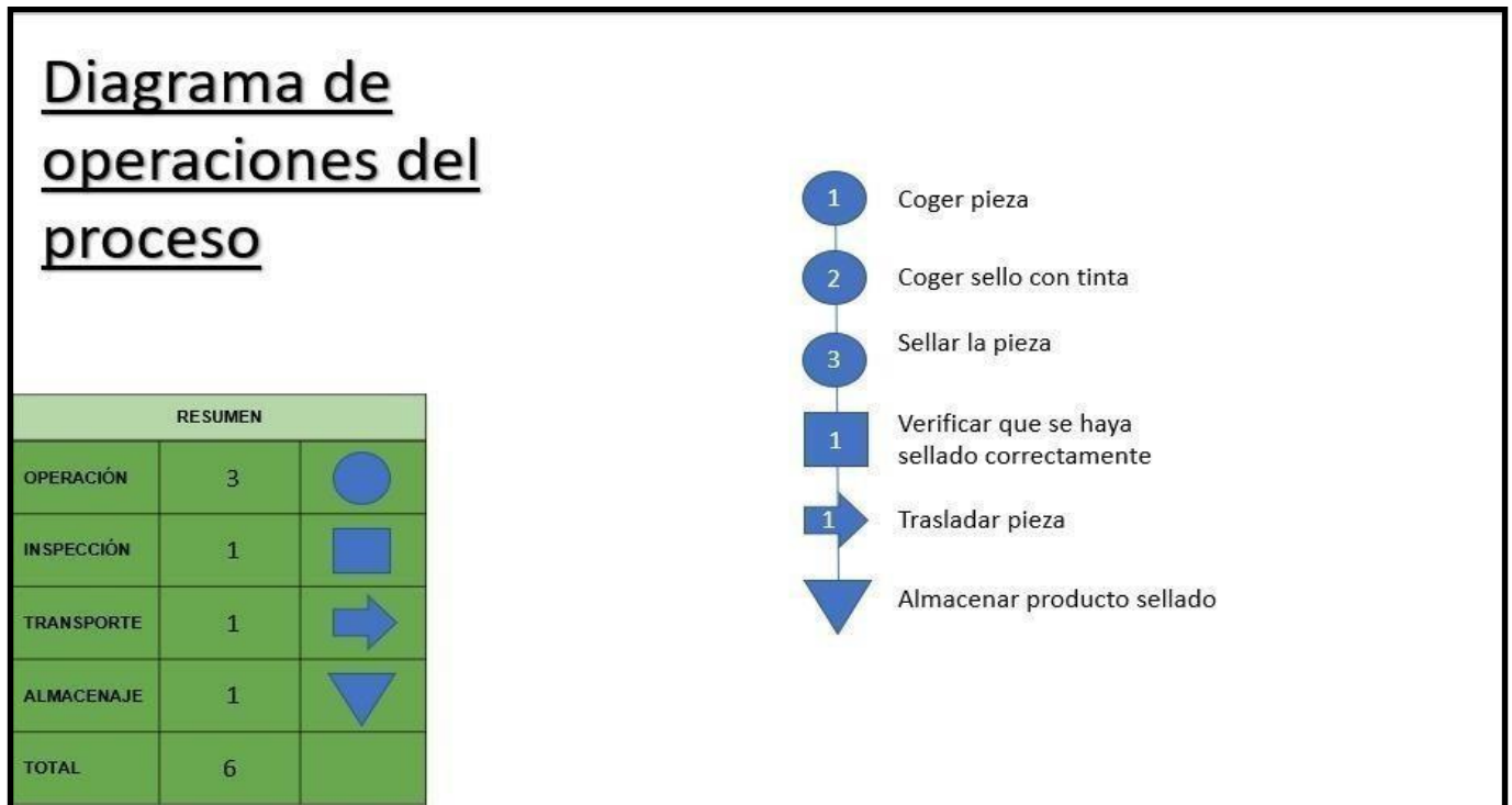
Fig. 13. Diagram of operations of the current process for sealing.
