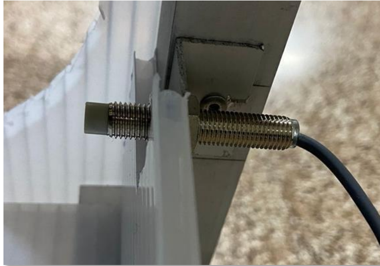
Figure 05: Inductive Sensor Source: Own elaboration
