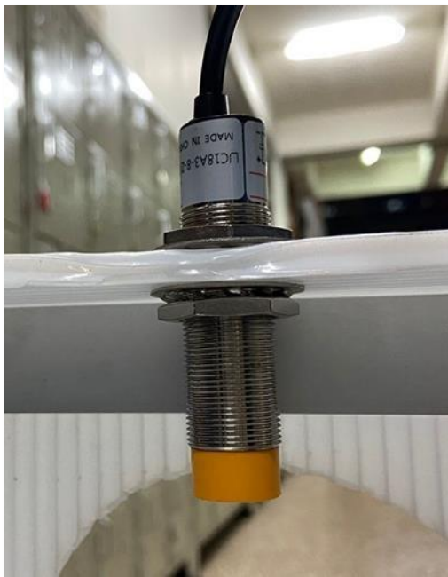
Figure 06: Capacitive sensor Source: Own elaboration
