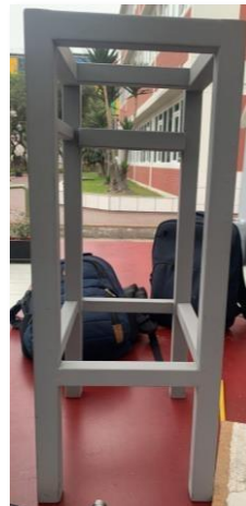
Figure 16: Galvanized iron structure Source: Own elaboration
