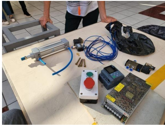
Figure 25: Components for the elaboration of the project: PLC, Piston, Power supply, pushbutton panel and solenoid valves.
