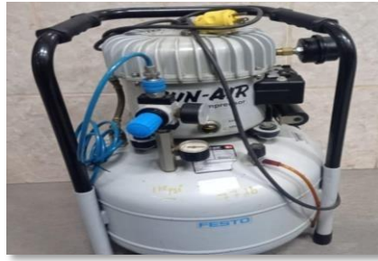
Figure 14: Compressed air compressor Source: Own elaboration
