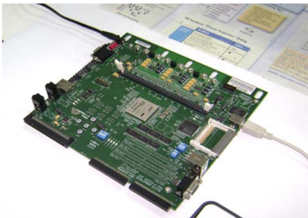
Figura 8. Board XUP2VP30 of XILINX.
