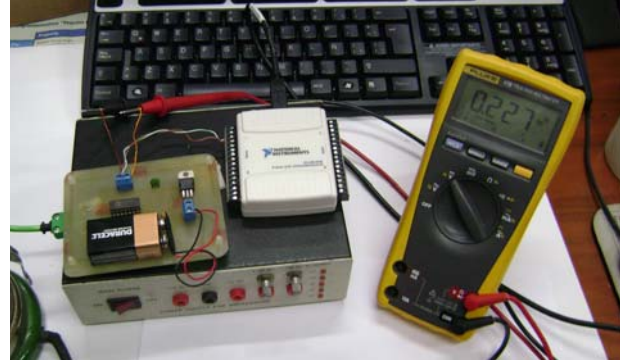
Figure 18. Connection between DAQ and Signal conditioner.
